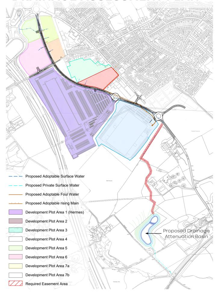
The Western catchment collects approximately 16.55 hectares of Hoyland West; this is currently funnelled into Harley Dike. As this outfall is proposed to be the primary outfall for the development, greenfield runoff calculations have been done, to ensure that proposed runoff rates resulting from the development are not greater than those currently experienced. Early calculations suggest that approximately 43,000 square metres of drainage attenuation is required.
