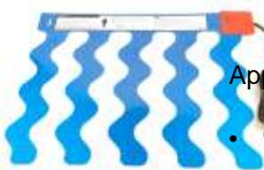
Application - generates an alarm when tonic-clonic seizures are detected in bed.
