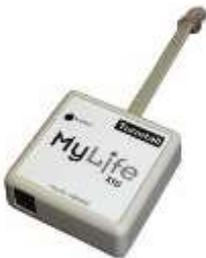
Application – provides the Lifeline Connect+ with ability to switch devices on/off such as lights using the X10 main and secondary controllers.
