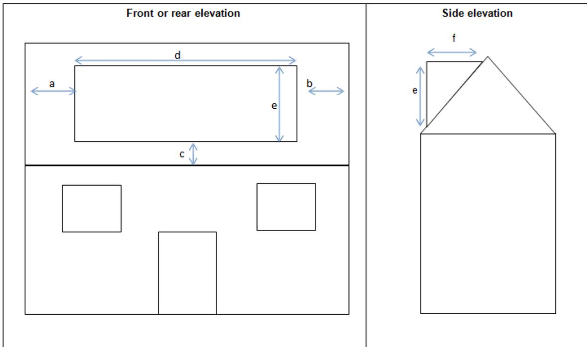
Example sketch plan (guidance on where to take measurements from)
