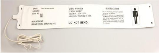
Raises a call if service user is out of bed longer than a reasonable time period. Can also be set to raise an alarm if not in bed by or out of bed by a defined time. Switches on a bedside light when getting up during the night and switches off when return to bed.
