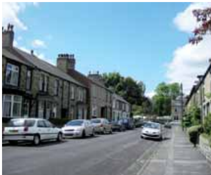
This street has a ratio of about 1:2 and gives a comfortable degree of enclosure
