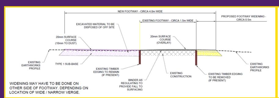
Pictured on the left is a cross section of the route design which will be applied to the majority of the route.
